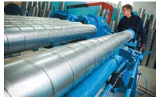
Spiral air ducts workshop
