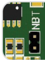
Figure 5. Mains bus resistor jumper
