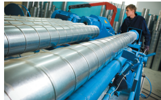
Spiral air ducts workshop
