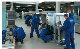
AirVents air handling unit workshop
