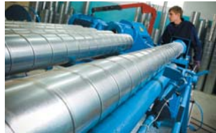
Spiral air ducts workshop
