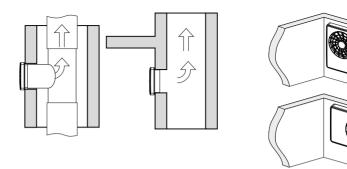
The replaceable adapter of required size may be used to facilitate mounting.
