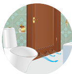
Bathroom / door intake grille
