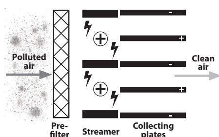
The filter cleaning interval depends on the inlet air pollution density and may vary from 7 up to 21 days.
