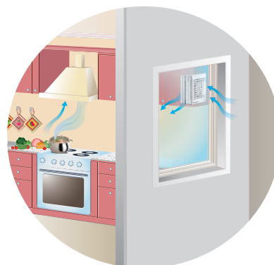
Fan operation in reverse SUPPLY-EXHAUST mode
