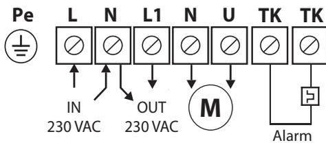
Controller wiring diagram
