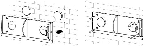
Install the front part of the hood and fix it with screws.
