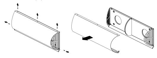
Mark the holes using the back part of the ventilation hood. Drill 4 holes for the dowels.
