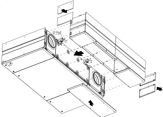
Install the decorative panels. Install the panels in the centre first, then the top and bottom panels. Special fasteners are used to mount the unit with the product. Mounting brackets for mounting the unit with the product are included with the unit.
